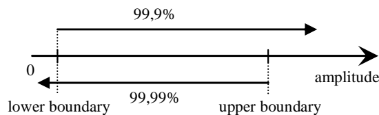
Fig. 4. Defining lower and upper boundary of amplitude range that will be displayed
