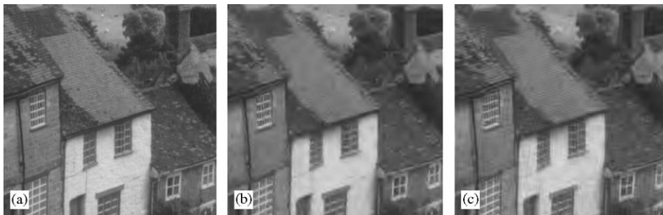
Fig. 11. Magnified detail from image Goldhill: (a) original, (b) SPIHT decoded, 0.25 bpp, (c) WP-SPIHT decoded, 0.25 bpp.
