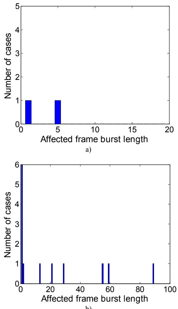
Figure 2. Histogram of affected frame length versus number of cases, UC3D database, video 1 (balloons): a) best case (AFR= 2%), b) worst case (AFR= 91.33%)
